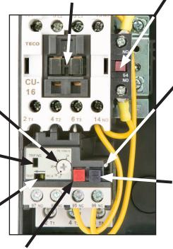
**ON Button:** When pushed, power is sent to the magnetic field coil, closing the contactor and sending power to the motor.
